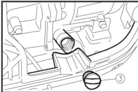
4. Fill the specified amount of the recommended engine oil, and then install and tighten the oil filler cap.
