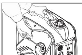
5. After the engine starts, warm up the engine until the engine does not stop when the choke knob is returned to the ~~⑤~~ ④ “ON” position④.
