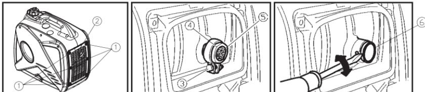
2. Loosen the bolt ③ and then remove the muffler cap ④, the muffler screen ⑤ and spark arrester ⑥.
