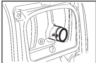
6. Install the muffler screen and the muffler cap.
