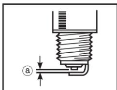
**TIP:** The spark plug gap should be measured with a wire thickness gauge and, If necessary, adjusted to specification.
