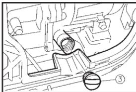
4. Place an oil pan under the engine. Tilt the generator to drain the oil completely.
