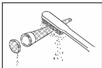
4. Check the muffler screen and spark arrester. Replace them if damaged.
