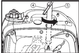
2. Insert the handlebar ④ into the tool ⑤ and turn it counterclockwise to remove the spark plug.
