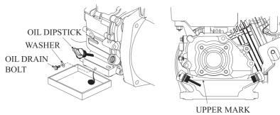
4. Reinstall the oil dipstick and tighten it.
