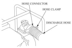
It is best to use a short, large-diameter hose, because that will reduce fluid friction and improve pump's output.
