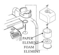
Screw off butterfly nut and remove air filter housing, If the element is
