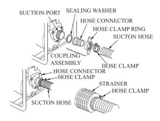
Hose dimension should be longer than water suction port dimension. Minimum hose dimension shall be as following: 2" water pump 50 mm
